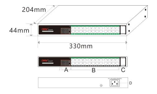
A.Working indicator B.24\*PoE ports C.2\*1000M uplink SFP ports D.power input portAC100-240V,50-60Hz
