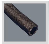
Style 7810 is a firm, high density, non-asbestos packing. It can handle steam, most chemicals, mild acids, and alkalies. It is excellent for use in steam turbines, high temperature motoractuated slide valves, and in high pressure/high temperature valving in general.
