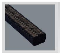
Chemically inert over the entire 0–14 pH range with these exceptions: molten alkali metals, fluorides, oleum, fuming nitric acid, aqua regia, and other strong oxidizing agents. An excellent general service and corrosive service packing. It is commonly used in pumps, in valves, in rotating and reciprocating shafts, in mixers and agitators, and is especially designed for services involving surface speeds and temperatures higher than
