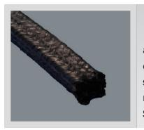
Style 7830 packing is ideally suited for use in severe service valves and rotary shaft applications. It handles strong acids and alkali solutions except fuming nitric acid, oleum and fluorine. It can be used to seal steam, water, oil, solvents, alkalies, and acids. It is often used as end rings for packing sets utilizing softer packings that might tend to extrude. Style 7830 also handles high temperatures, extremely high shaft speeds
