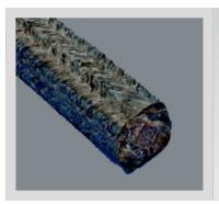
Style 7603 packing can handle chemicals over the entire 0–14 pH range except for strong oxidizers. It is very popular in the pulp and paper industry because it is especially designed for applications involving strong caustics, acids, bleaches, slurries, and services where contamination cannot be tolerated. Style 7603 is commonly used in valves and pumps, agitators, reactors, and autoclaves.
