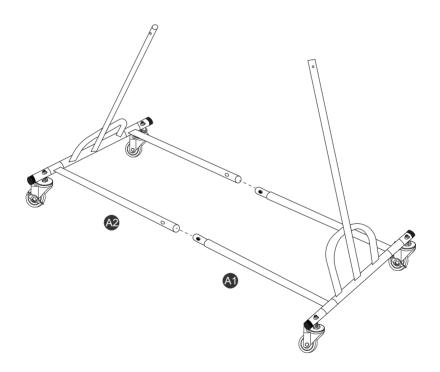
Step 4 Insert part (B) into part (A)&A2), as shown above.
