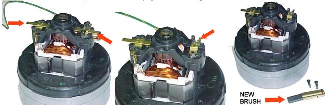
Figure 3 - Brush casings and screws
