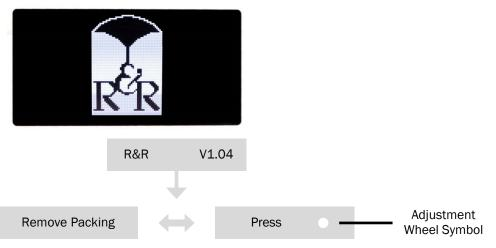
The display shows the "Remove Packing" reminder and alternately the "Click To Continue" command.
