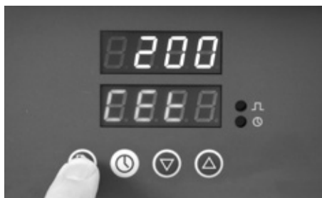
End temperature at which the furnace may be opened. Here: 200°C (default setting)
