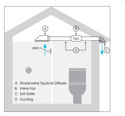
The Shadowline Diffuser Squircle requires a circular ceiling cutout (refer to dimensions drawing). The diffuser should be installed prior to the ceiling being installed, as the plenum box is larger than the ceiling cut out. Please check product specifications with your tradesperson before ordering.
