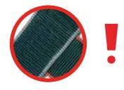
If structural sewing is missing stop use and contact DMM:
