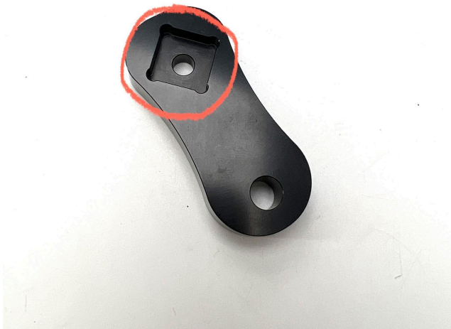
The square recess should fit the marked part of the lever
