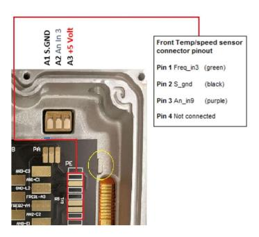
Start by connecting the supplied 3 pin DTM to the 3 wires marked with 4, 5 and 6. Use protective sleeving around the wires.
