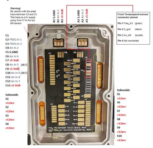
Install the PCB inside the mechatronics module using high temp RTV.
