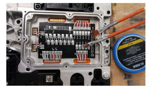
Tin pads and wires (use flux paste) and then solder the wires to the pads.
