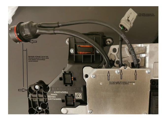
Note that the cables are not marked, but have color coding to identify its usage. Positions of **solenoid 1-10**, **An\_in 1-9**, and **Freq\_in 1-3** are set by the end user.
