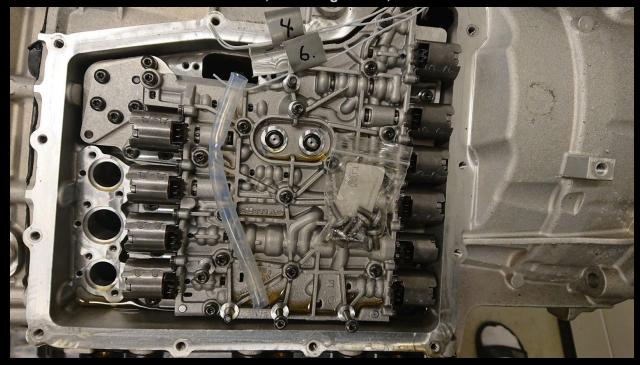
Inspect shift fork holes 3x to the left and torque/speed sensor hole on middle top. Most likely there are metallic debris down there that can be cleaned with a Q-tip/cotton swab. Close up the mechatronics cover and seal the hole for the gearbox connector.
