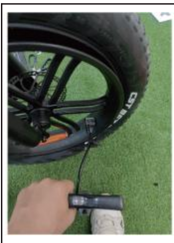
17. Fill the tires with air.
