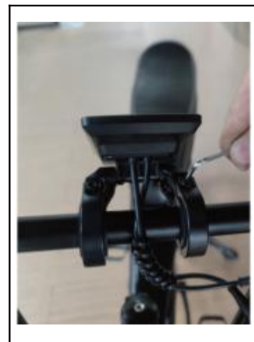
18. Install the dashboard and tighten all screws.
