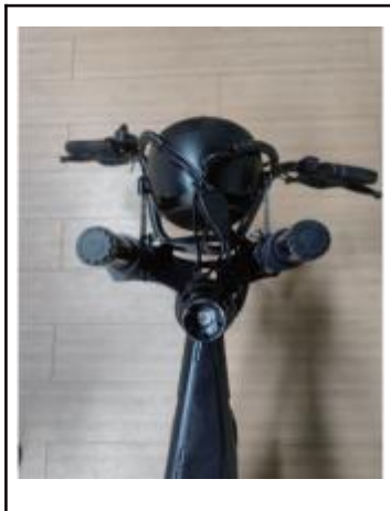
7. Put the steering in front.
