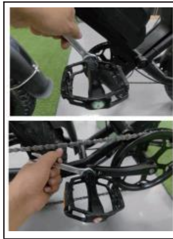
16. Install the pedal and tighten the screw.
