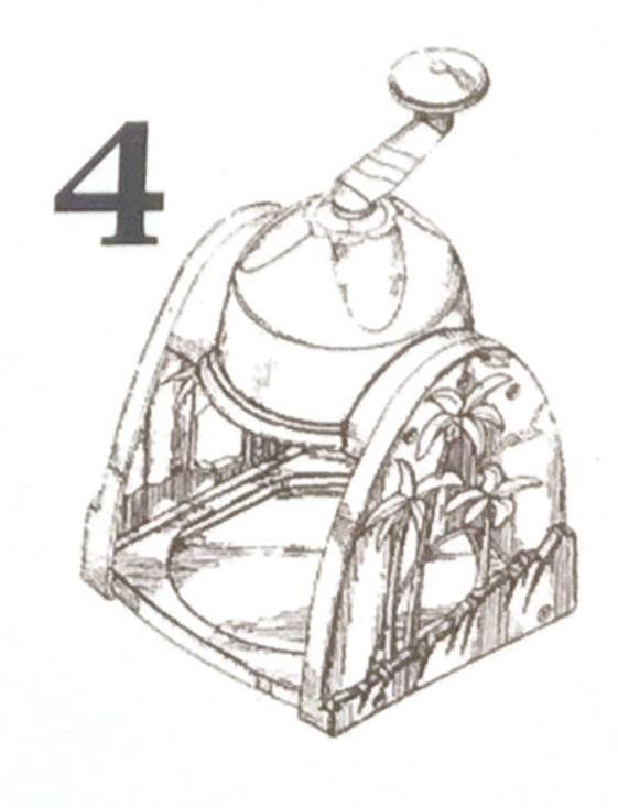
Fix it by pressing the cover with one hand. Then turn the handle clockwisely for cutting ice.
