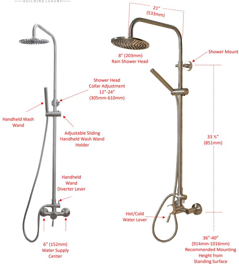
Shower is supported by single mount at top. Requires secure plumbing at water supply inlets to prevent shower from swinging outwards.
