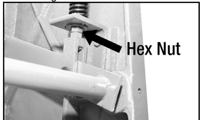
Figure-9 Return spring tension
