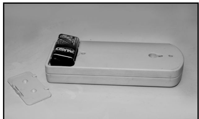
Figure-7 Replacing remote control battery
