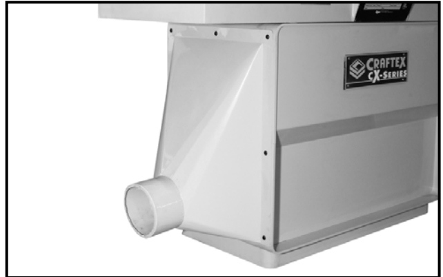
Figure-5 Installing the dust hood
