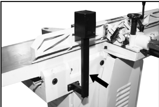
Figure-3 Installing the switch bracket
