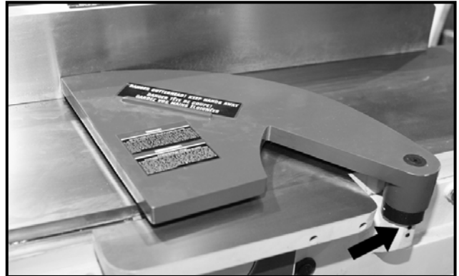
Figure-4 Installing the cutterhead guard
