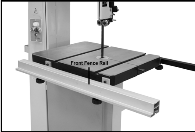
Figure-12 Front fence rail installed
