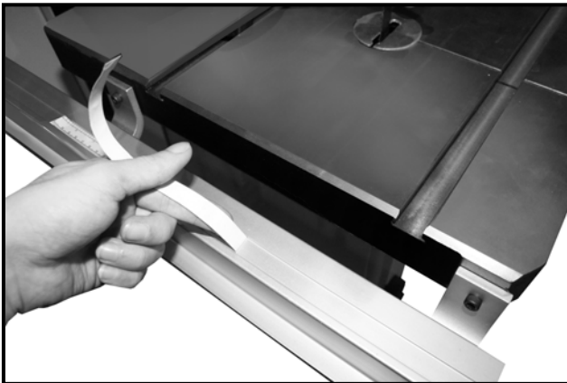
Figure-13 Adhesive backed scale attached to the front rail
