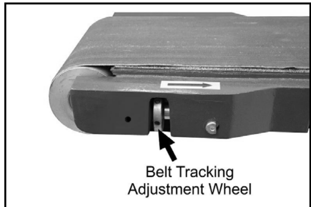
Figure-6 Belt tracking adjustment wheel
