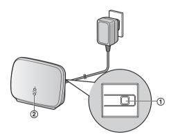
The indicator lights when the registration is completed. (Depending on the signal status, the indicator may not light in green. In this case, see the repeater's Getting Started.)
