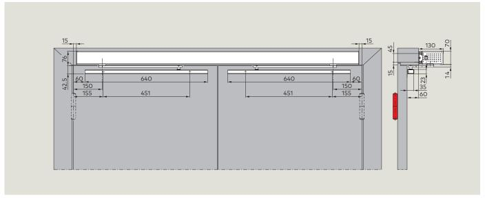
The push-version with slide channel is not suitable for smoke control doors and fire doors
