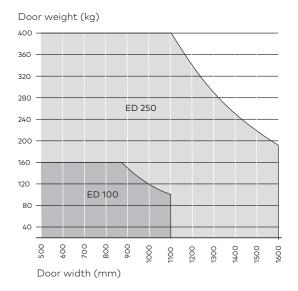
The drives ED 100 and ED 250 are suitable for most swing doors provided that the combination of door width and door weight lies within the defined functional area.
