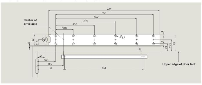
View: BASIC cover, push-version, 12.5 mm pivot pin, standard axle extension
