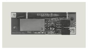
The BRC-R radio receiver may easily be installed inside the drive as its size is adapted to the available space. Simply fix it on the motorgear-unit with two screws.
