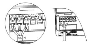
③ Properly connect the AC output wire according to the wire sequence and terminal position shown in the figure below. Please connect the ground wire first, and then the live wire and the neutral wire. The ground wire is connected to the grounding screw hole on the cabinet through the O-type terminal.
