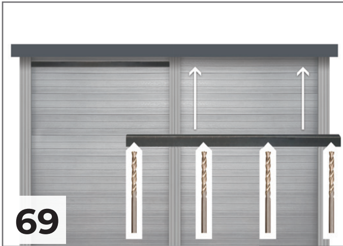
69 Pre-drill 4-5 holes (using a 3mm drill bit) in the BT1 trims and fix them to the back wall between the posts. (approx. 60mm below the top edge of the wall panels).
