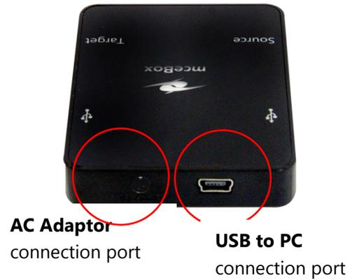
2. Connect one end of the supplied USB-to-PC connection cable to the back of the Connection Hub and the other end to an available USB port on your PC.
