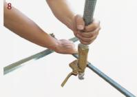
Adjust the positions of the center bracket and the flexible hose to desired location.
