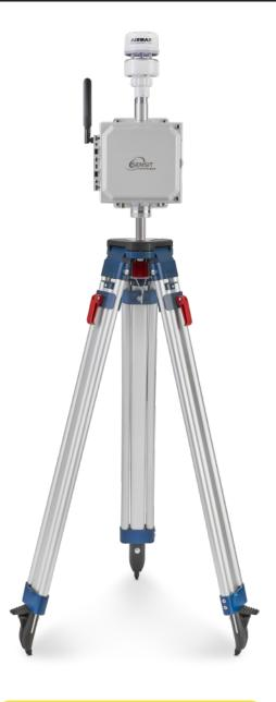
The **SENSIT**® **SPOD** is a low-cost, solar-powered sensor system that combines wind and air pollutant concentration measurements to detect VOC emission plumes and help locate the source of emissions.
