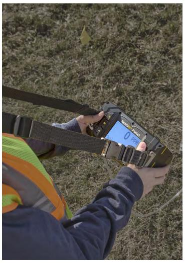
The **SENSIT® PMD2** is a small, lightweight precision instrument used to survey, pinpoint, and grade methane leaks. With TDLAS technology, the **SENSIT® PMD2** is methane selective and perfect for walking or vehicle applications.
