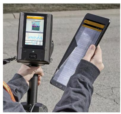
The GAS•TRAC® LZ-50 is an innovative handheld methane gas detector that provides instantaneous readings from a distance to the target of up to 164′. Its revolutionary laser photonics combined with breakthrough technology, TARGET PS, makes it the clear choice in remote laser methane detection.
