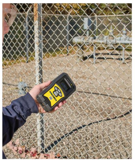
The **LZ-30** from SENSIT Technologies is a compact methanespecific leak detector that provides fast and accurate readings at distances up to 100 feet.
