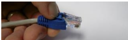
Pull boot back to access lock clip
