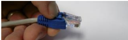
Pull boot back to access lock clip
