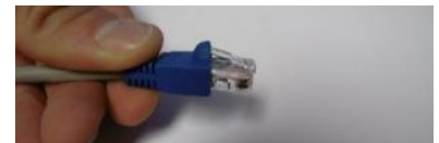
Slide boot back over lock clip
