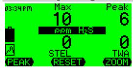
During peak mode (activated by pressing the left key PEAK), peak values can be monitored and displayed. The display shows an animated symbol in the bottom left corner.
