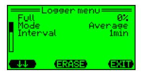
If **Interval** is selected, the data recording interval can be set between 1 second and 60 minutes by pressing and and
