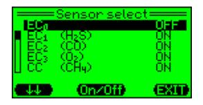
ON or OFF indicates the status of the sensor (active or inactive).
