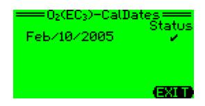
Within the sensor menu point Calibration dates, the date of the last calibration can be displayed, as well as if the calibration was successful  $(\sqrt{})$  or not  $(\cancel{\times})$ .
