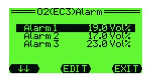
After selecting the sensor menu point Alarms the following reading is displayed (here, for an O<sub>2</sub> sensor):
