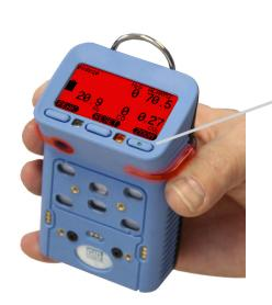
Turn the G460 on in an environment known to be free from gases and / or vapors.
