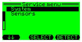
Select Sensors to adjust sensor-specific functions (alarms, calibration, etc).
