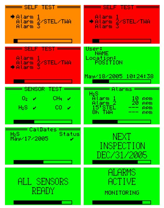
**NOTE:** GfG recommends that you "bump check" the sensors before each use to confirm their ability to respond to gas. To do this, expose the detector to a gas concentration that exceeds the alarm set points. Manually verify that the audible and visual alarms are activated. Calibrate if the readings are not within the specified limits.
