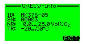
Type of sensor (ID) Serial number (SN) Detection range (NR) Temperature range (TR) -**Temperature**
