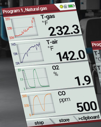
Flue gas Measurement screen with graphics
