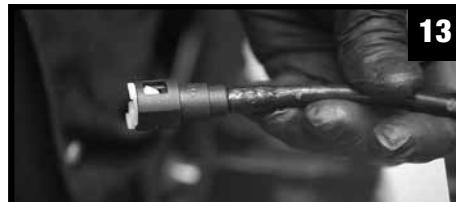
For 90° quick-connectors, the procedure is the same except that instead of the quick-connect insert, you will use the 90° quick-connect holder:
