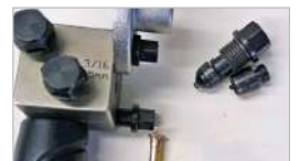
STEP 4: Remove die head. Loosen block. Inspect flare.
