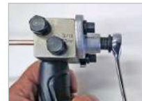
STEP 3: Insert OP2 flare head into die block. Tighten with a 12mm wrench or socket.
