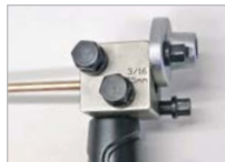
STEP 1: Insert tubing, set depth, and tighten.
