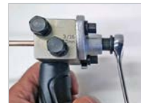
STEP 3: Insert OP2 flare head into die block. Tighten with a 12mm wrench or socket.
