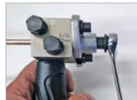
STEP 2: Insert OP1 flare head into die block. Tighten with a 12mm wrench or socket.
