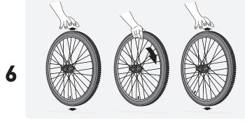
Bounce: Hold the wheel vertically and gently bounce or "dribble" it to disperse sealant throughout the inside of the tire. Let the wheel drop from an inch or two, then rotate a few degrees and repeat. Do this for several revolutions of the wheel.
