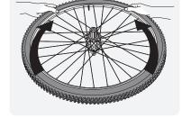
Mount tire: Making sure to position the tire bead in the center channel of the rim, mount one tire bead beginning opposite the valve and finishing at the valve. Once the first bead is mounted, begin mounting the second bead opposite the valve and finish at the valve.
