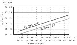
Inflate to riding pressure; the chart above is a recommended starting point. Always review the maximum pressure information listed on both the rim and the tire and consider the lower of the two numbers your maximum pressure. Do not inflate above the lower of the two numbers.
