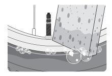
With a brush or sponge apply a generous amount of soapy water to both beads of the tire to help it slip onto the bead of the rim when inflating.
