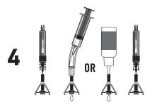
Add sealant: Once successful with inflation remove the valve core to add Stan's sealant. Add 2–4 oz. of sealant.
