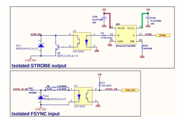
**External Triggering:** Sensors require 1V8 rising edge on FSYNC for the trigger event. We are using an optocoupler and ESD protection diode, so the input trigger voltage should be 12V (up to 24V) and the trigger logic is reversed, so trigger event happens at 0V on the FSYNC line. For example, see <u>External FSYNC Example</u>.
