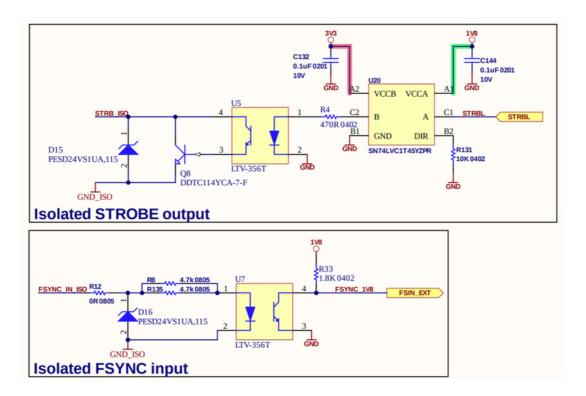
**External Triggering:** Sensors require 1V8 rising edge on FSYNC for the trigger event. We are using an optocoupler and ESD protection diode, so the input trigger voltage should be 12V (up to 24V) and the trigger logic is reversed, so trigger event happens at 0V on the FSYNC line. For example, see <a href="External FSYNC Example">External FSYNC Example</a>.
