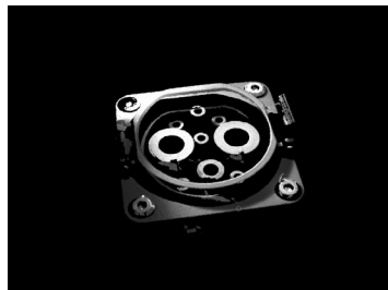
Car Charging Port
