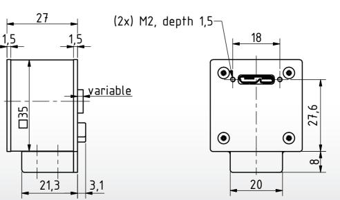
Dimensions: mm Tolerances: DIN ISO 2768m
