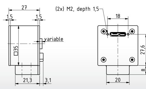
Dimensions: mm Tolerances: DIN ISO 2768m
