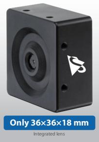
The Imaging Source DFK AFU050-L34 color camera has a USB 2.0 interface and is the perfect solution for many industrial automation, quality assurance, security, surveillance and medical applications. With up to 60 images per second, the DFK AFU050-L34 is a low cost, yet highly versatile imaging solution. The camera integrates an autofocus lens (One-touch)
