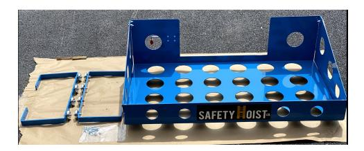
2. Bolt a **deck extender** into pre-existing mounting holes on the side of the carriage using the nuts and bolts provided and secure. Repeat the step on the opposite side of the carriage. Please note, side skate wheels (2) must be removed to complete this step. Skate wheels can be reinstalled once assembly is complete.
