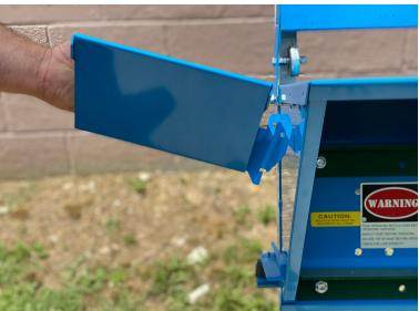
3. Place **Utility Tray L** on the top of the carriage and align with the (2) pre-existing deck extender mounting holes per side.
