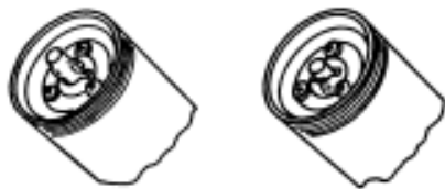
UNLOCKED LUGS PARRALLEL TO SLOT
