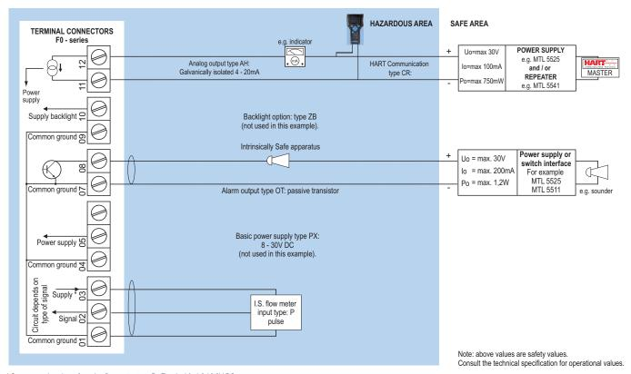
$<sup>^{\</sup>star}$  Sensor supply voltage for pulse flow meter type P : Terminal 3: 1.2 / 3.2V DC.
