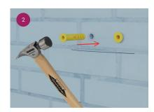
Hammer in the provided masonry wall anchors.
