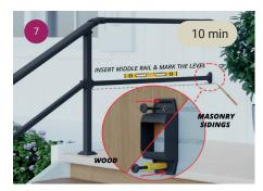
Insert the middle rail into the bracket, mark the horizontal position on the wall (use a leveler) and install the wall bracket for the middle rail (for drilling instructions, please refer to the 'Drilling Guide' on the other side).
