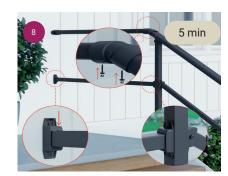
Secure rail using self-drilling screws provided. For top rail connector, use 2 screws on each end on the bottom side. For the middle rail bracket, use 1 screw on the narrow side. Screw in tight enough where the screw-head meets the metal.
