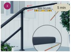
Insert the top rail into the connector, bring it down to horizontal position (use a leveler) and mark the position of the bottom of the rail on the wall with a pencil.
