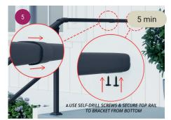
Insert the top rail, slide the wall connection cover into the rail (thin side facing in) and let the handrail rest horizontally on the wall bracket. Now, insert two self-drilling screws through the wall bracket and into the handrail to secure it in place.
