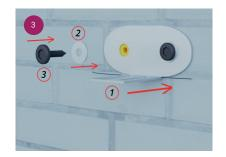
Using the screws provided with the masonry wall anchors, put a washer onto the screw, and secure the bracket in place.
